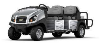
Payload: Total vehicle capacity of 1,500 lb. (680.3 kg).
